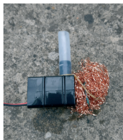
Copper mesh used as filter.
