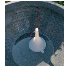
Use a funnel as a base for the pipe. The pump sits within it.
